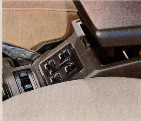
Centre console houses controls for electric windows, headlamp washers and rear window wash and wipe.
