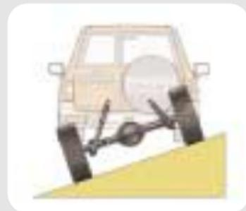
The switchable stabiliser gives you the best of both worlds. Select "OFF" and the rear anti-roll bar disengages to give you maximum axle articulation for tackling the most arduous off-road conditions. Switch to "ON" and you have the ideal set-up for predictable handling and optimum on-road stability.
