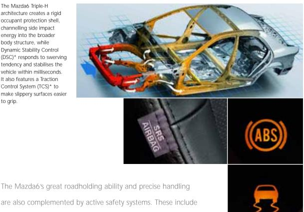
are also complemented by active safety systems. These include Anti-Lock Brakes (ABS) with Electronic Brake-force Distribution (EBD) that adjusts the braking force to suit the handling, and Dynamic Stability Control (DSC)\* with Electronic Braking Assistance (EBA) and Traction Control System (TCS)\* to give you extra control on slippery surfaces.
