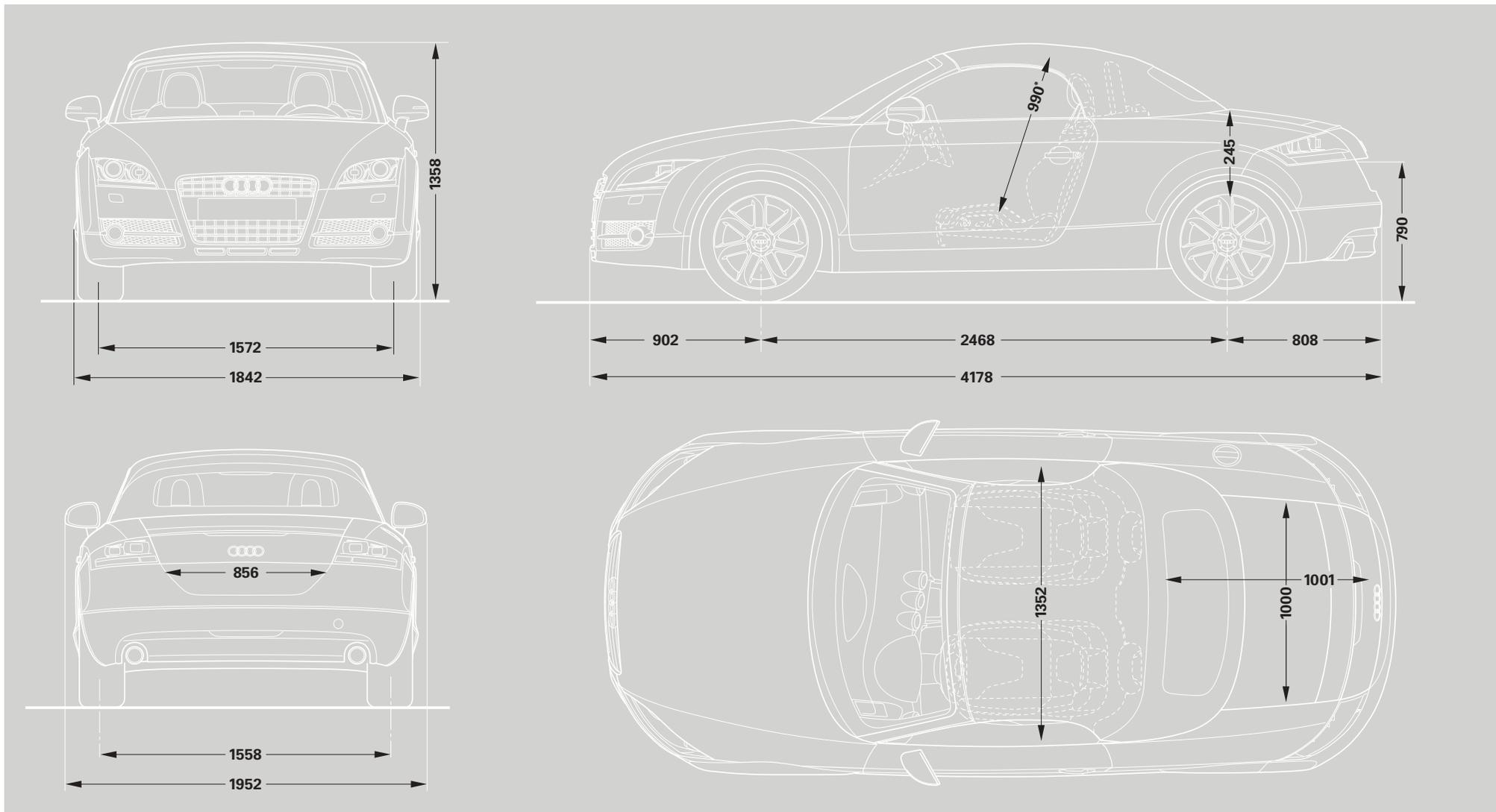
Dimensions were measured at unladen weight. Luggage compartment volume 250l (measured in accordance with the VDA method using 200 x 100 x 50mm blocks)
