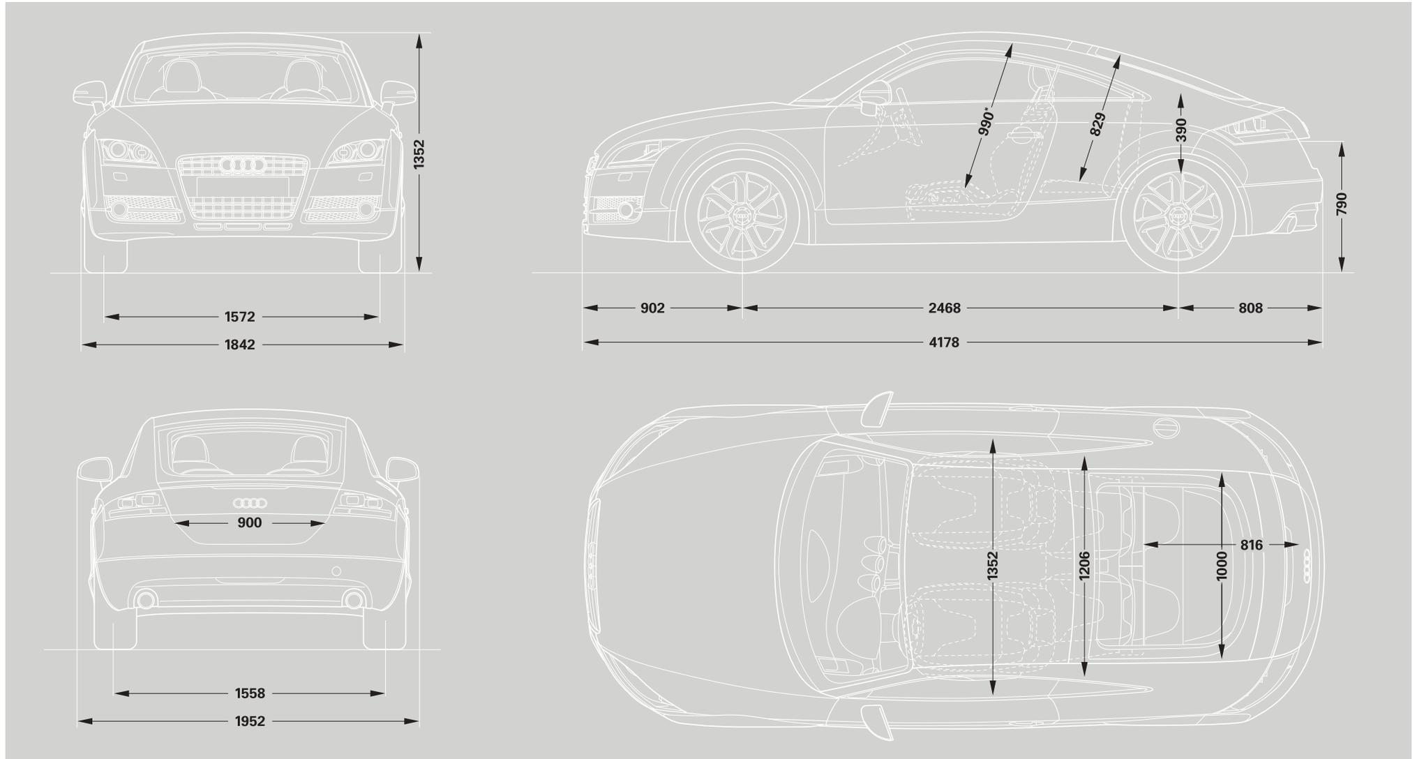
Dimensions were measured at unladen weight. Luggage compartment volume 250/700l (measured in accordance with the VDA method using 200 x 100 x 50 mm blocks; second figure: with rear seat folded down and the vehicle loaded up to roof height). Turning circle approx. 10.9m. \*Maximum headroom.
