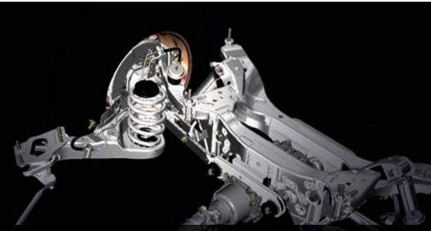
Independent rear multi-link suspension allows secure cornering and ensures stability at high speeds.
