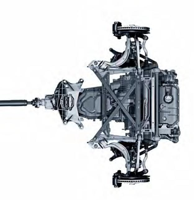
In the A5 Coupé, asymmetric dynamic torque distribution continuously distributes drive power between the front and rear axles, depending on weather conditions, road surface and gradient. This leads to greater flexibility and an enhanced, sportier drive.
