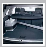
Load-securing set with rails
