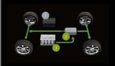
While driving at low speeds or in start-and-stop traffic, the vehicle may operate fully in electric mode.
