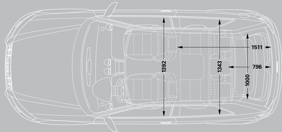
Dimensions were measured with vehicle at unladen weight.
