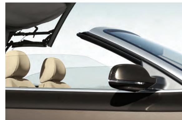
Exterior mirrors – electrically operated and heated
