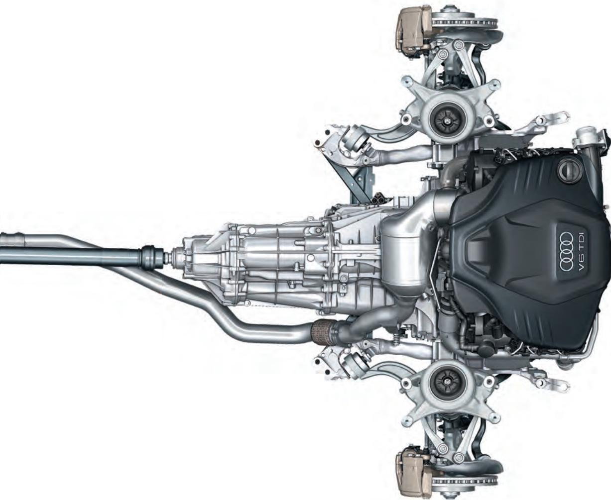
In the Audi A5 Cabriolet, asymmetric dynamic torque distribution continuously distributes drive power between the front and rear axles, depending on weather conditions, road surface and gradient. This leads to greater flexibility and an enhanced, sportier drive.
