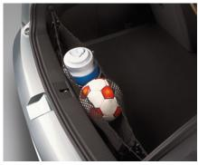
This flexible cargo net can be installed in two different positions. Azip on each side of the cargo net allows you to choose the position that works best to help keep items from shifting in the cargo area of your Volt.
