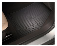
FLOOR MATS - PREMIUM (ALL WEATHER) Premium All Weather floor mats feature a custom deepribbed pattern to collect rain, mud, snow and debris. Nibs on back help hold mats in place and conform to the floor of your Volt. Front mats feature the Volt logo. Set of 4.
