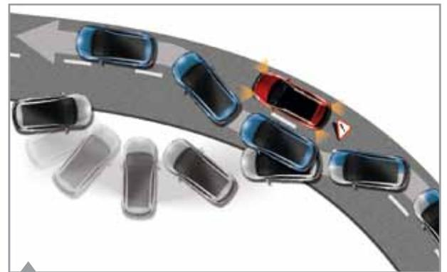
**ESC (Electronic Stability Control)** - if a loss of grip is detected, ESC applies the correct amount of brake pressure to each individual wheel, helping you maintain control and stability. It also reduces engine power to help you maintain control.
