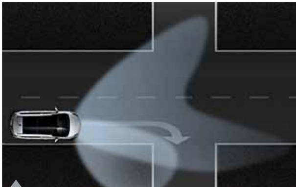
**Cornering lights** - When driving at night the cornering lights automatically turn on to illuminate potential hazards when turning.
