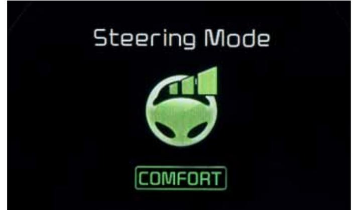
**Flex Steer** - This innovative feature allows you to choose between three modes of steering - simply select 'comfort' to make light work of city driving, 'normal' for regular driving or 'sport' mode for even more responsive steering, ideal for motorway driving or on narrow country lanes.
