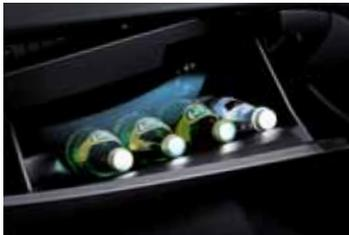
**Cooled glove box** – The 8-litre glove box has a cooling function, handy for chilling drinks or storing perishable items on longer journeys. It is illuminated for convenience especially at night.
