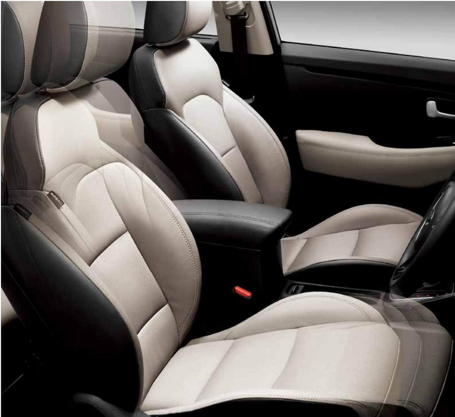
**10-way power adjustable driver's seat ('3' grade)** - The driver's seat can be adjusted up to 10 ways as it electrically tilts, slides and reclines plus it boasts electric lumbar and height adjustment settings too. (Beige leather upholstery shown is available on the Powder Blue exterior colour only)\*
