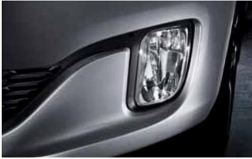
**Front fog lights ('2' upwards)** – integrated into the front bumper, the fog lights combine safety considerations with aesthetic appeal.
