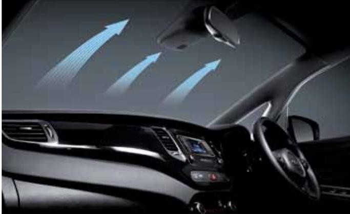
**Auto de-fogging system ('2' upwards)** - A sensor automatically initiates a de-fogging process when condensation is detected on the windows to ensure optimal visibility and to prevent humidity from building up on the windows.
