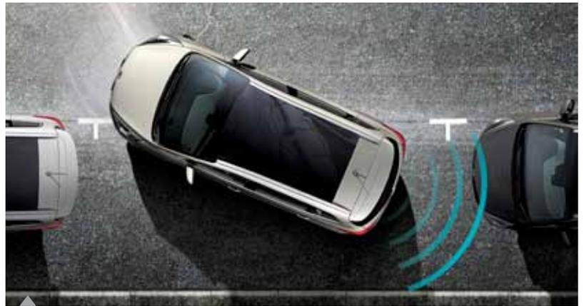
**Reversing camera integrated into the centre fascia screen ('3' grade)** – The popular reversing camera feature is combined with reversing sensors which help minimise the collision risks involved when parking or manoeuvring. The rear camera view shows superimposed parking guidelines to assist the driver in easier, more effective parking.
