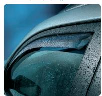
**Side window wind deflector, front only** Reduces turbulence and wind noise when driving with a slightly open front window. The aerodynamic shape redirects airflow and raindrops.
