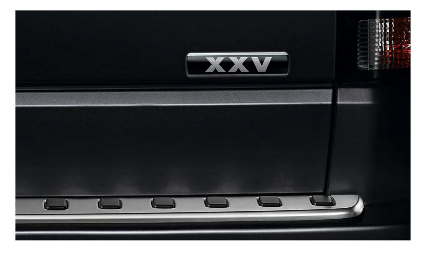
At the rear of the vehicle, a stainless steel tread plate is both functional and stylish. Whilst on the tailgate, the XXV ingot adds another unique touch.
