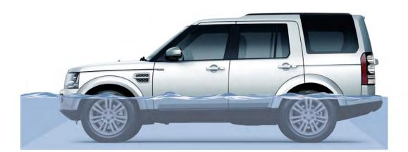
Width 2,053mm mirrors folded Width 2,200mm mirrors out
