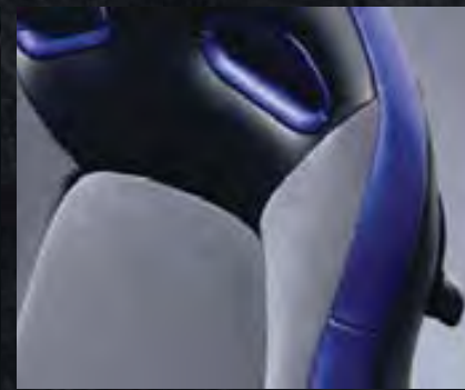
Track Pack seats are made from high grip material designed to keep the driver in place under heavy cornering
