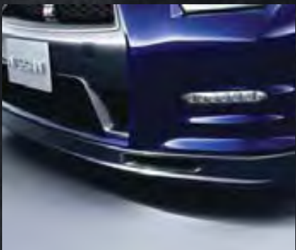
The reinforced brake cooling system decreases temperatures upto 100 degrees
