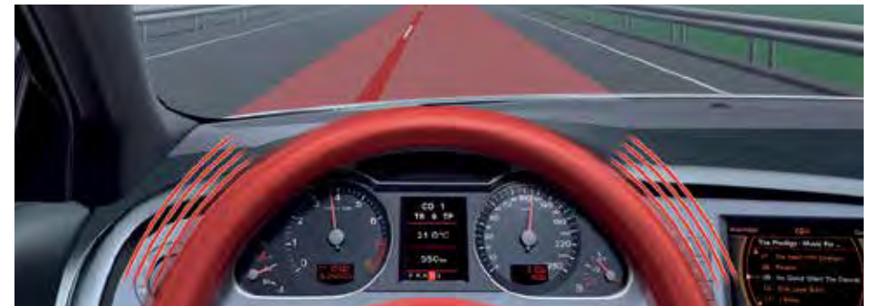
Audi active lane assist – steering wheel vibration
