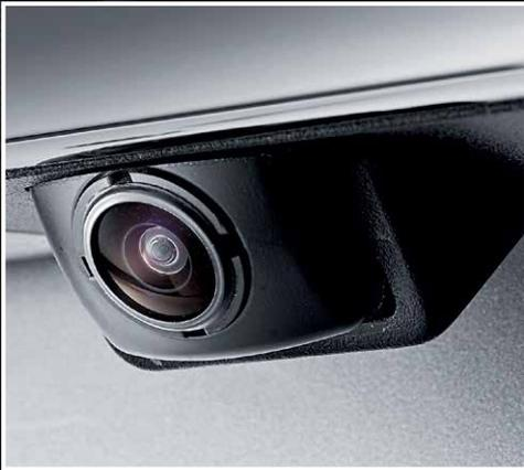
**Reversing camera integrated into the centre fascia screen ('3' and '4' grades only)** – The popular reversing camera feature is combined with reversing sensors which help minimise the collision risks involved when parking or manoeuvring. The rear camera view shows superimposed parking guidelines to assist the driver in easier, more effective parking. Reversing sensors are a standard feature on the new special edition 'SR7' models upwards.
