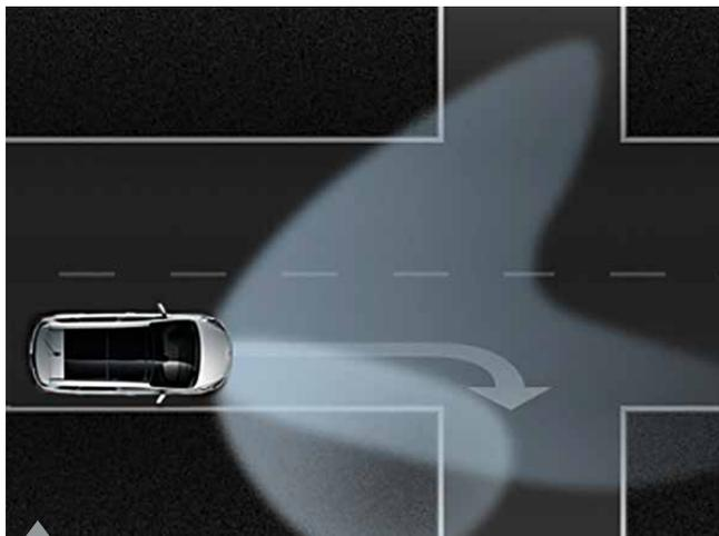
**Cornering lights** - When driving at night the cornering lights automatically turn on to illuminate potential hazards when turning.
