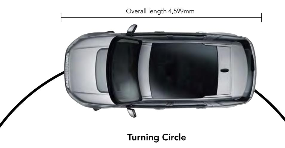
Kerb-to-kerb 11.6m Wall-to-wall 11.86m Turns lock-to-lock 2.31
