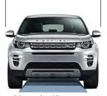
Obstacle Clearance Standard ride height 212mm
