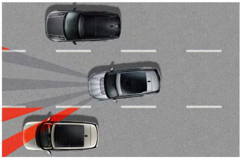
A forward-facing camera mounted ahead of the rear view mirror monitors the lane markings on both sides of the vehicle and gives the driver a warning should the driver drift out of the lane without the indicators being triggered. The alert comes in the form of a discrete vibration through the steering wheel, allowing the driver to take the appropriate action.
