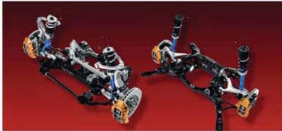
Handling duties are managed by a sophisticated four-wheel independent suspension system mounted to high-precision six-point front and rear subframes. A special Bilstein DampTronic driver adjustable shock absorber system utilises multiple vehicle information systems to provide appropriate damping forces and a high level of control for a variety of driving situations.
