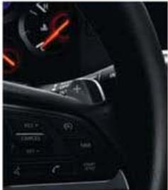
Two clutches. No clutch pedal. A lightning-quick shift. Inside Nissan GT-R's six-speed dual-clutch transmission, the clutches work together. When the car is in an odd-numbered gear (1st, 3rd, 5th), the even-numbered gear (2nd, 4th, 6th) is pre-selected and ready to make the shift immediately. The transmission is so smart, it even blips the throttle on downshifts to for smoother gear changes.
