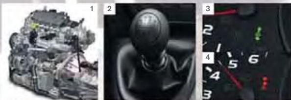
1) 2.3 LITRE DCI TURBODIESEL 2) SIX-SPEED MANUAL GEARBOX 3-4) GEAR SHIFT INDICATOR
