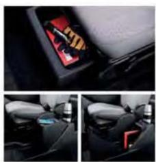
CENTRE CONSOLE is large enough to hold a laptop computer - it's even designed to hold hanging files.
