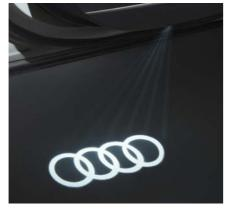
Audi Beam Projects the Audi rings on to the ground with LEDs when the door is open.
