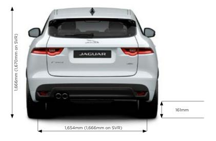
Dimensions were measured with vehicle at unladen weight.
