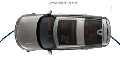
Turning Circle Kerb-to-kerb 12.4m Wall-to-wall 12.4m Turns lock-to-lock 2.7
