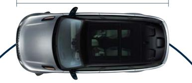
**Obstacle Clearance** Off-road height 248mm<sup>†‡</sup> Standard ride height 205mm<sup>+</sup>
