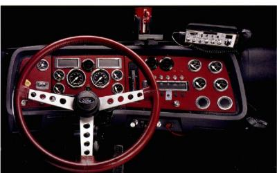
The driverfriendly instrument panel includes a dash-mounted beverage holder. CB radio platform and air suspension dump valve. Plus easy to read gauge clusters.
