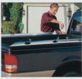
Attractive, sturdy pickup box rails feature specially designed tie-down loops that are excellent for securing loose cargo or tarpaulins. Rails are held in place by metal posts that mount in existing stake holes. Bright or black aluminum. Available October, 1992.
