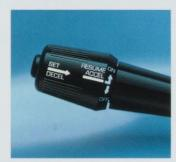
Speed control lets you sit back and relax as a microcomputer automatically maintains the cruising speed you choose. The unit disengages instantly when pressure is applied to the brake or clutch (manual transmissions) and returns to the original speed setting when the "resume" feature is activated.
