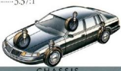
Body ..... unitized construction with separate front subframe Suspension: front: independent MacPherson struts with strut-mounted air springs, 19.0mm stabilizer bar, tension struts and lower control arms
