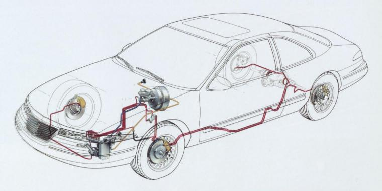
An adjunct to the ABS system which prevents wheel lock-up for safer stops, Traction Assist uses brake control to help prevent wheel spin.
