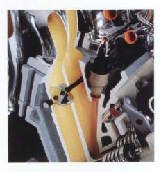
Separate air-intake runners feed each of the two throttle plates per cylinder, improving performance at all rpm.
