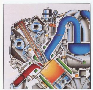
The lightweight, aluminumalloy cylinder head has hemispherical combustion chambers that maximize fuel efficiency and minimize emissions.
