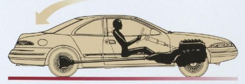
During acceleration, a car's weight shifts rearward. Unlike a front-drive model, traction on the Mark VIII is therefore increased. improving performance and driver control.
