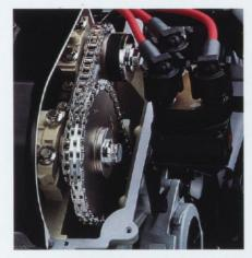
The chains that drive the camshafts are durable and operate quietly.
