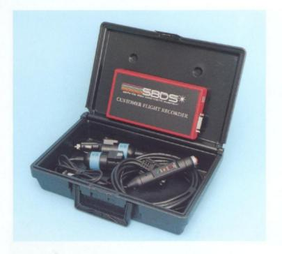
■ Service Bay Diagnostic System: Ford Motor Company has developed the Service Bay Diagnostic System<sup>®</sup>, or SBDS<sup>®</sup>. This system is one of the most important advances in the automotive service industry. It is a state-of-the-art, computerized, information and diagnostic system that helps technicians identify the cause of even the most difficult intermittent and hard-to-find driveability concerns.
