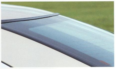
The one-piece molding is bonded to the rear window during manufacturing, and it is mounted to the body at zero tolerance, for a perfect fit and leak resistance.
