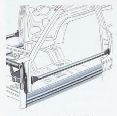
Door beams are made of ultra-high-strength, tubular steel.
