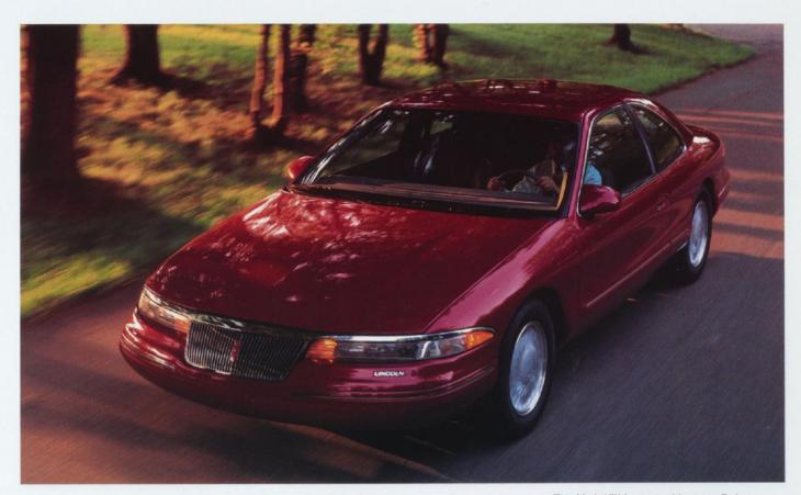
During acceleration, the car's weight shifts to the rear wheels, which are the Mark VIII's drive wheels. Increased weight on the drive wheels improves traction.
