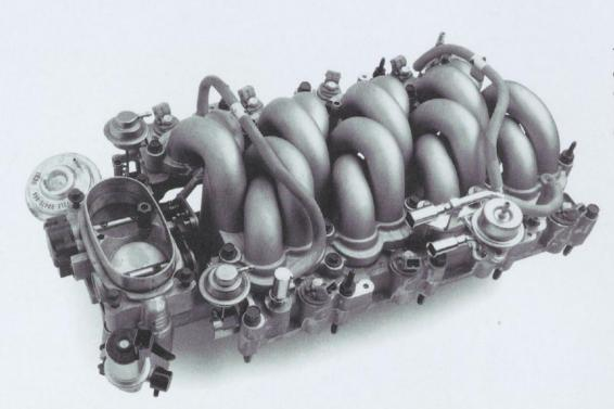
The intake manifold delivers cool air to the eight cylinders through 16 runners — two per cylinder.
