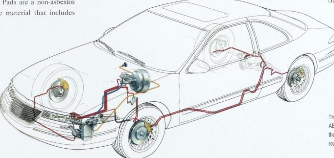
The four-wheel-disc brakes feature Teves ABS. An electronic-control unit manages the Traction Assist system, which uses the rear brakes to prevent wheel slip.
