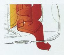
One-way vents allow interior air out of the car, for fresh-air replacement.
