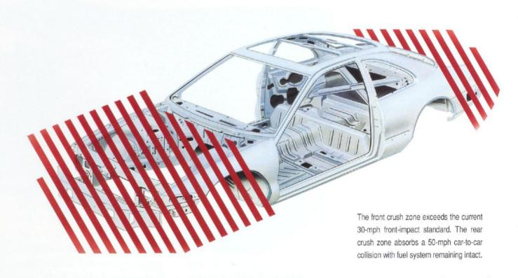
points and, if subjected to an impact, will collapse back at these points, rather than move rearwards into the windshield.
