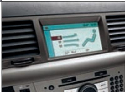
◀ **Electronic Climate Control (ECC).** Electronic Climate Control (ECC) allows you to select the temperature to the nearest degree and maintain it regardless of the outside temperature. The system, on some models, can even compensate for the effects of sunlight falling on one side of the car.
