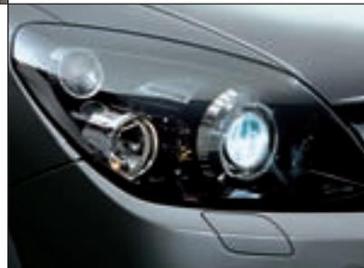
◀ **Adaptive Forward Lighting (AFL).** The optional lighting system swivels the beams up to 15 degrees for improved vision as you turn a corner. On some models AFL also raises the dipped headlight beam slightly at above 65mph, returning to normal beam automatically as speed is reduced.
