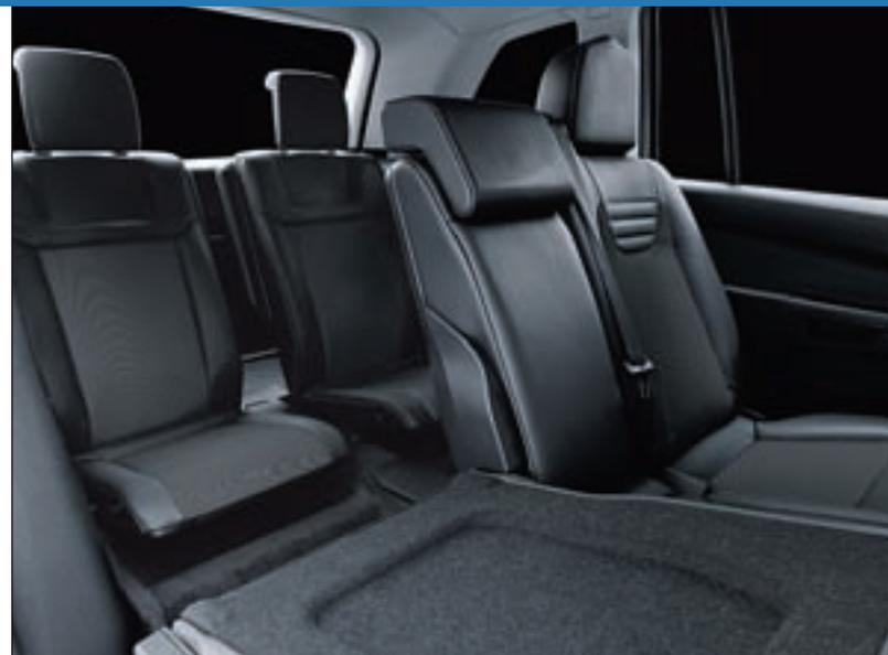
**Flex7® seating.** With Zafira's innovative Flex7® seating system, you can transform your VXR from a two-seater, high capacity carry-all into a spacious, seven-seater people carrier – and back – in seconds. When you're not using the third row seats, they can be folded flush with the load floor. So there's no need to remove them completely to free up luggage space. Both seats also fold separately, so you can accommodate six occupants plus a large item of luggage.
