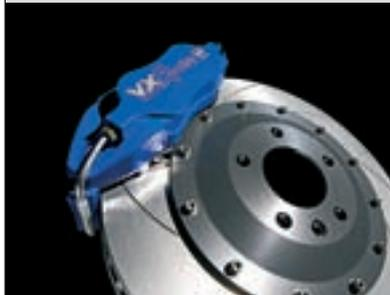
**▶ Braking systems.** For the driver who wants even more stopping power, VXRRacing have developed, with AP Racing, a front braking system using four-pot calipers with larger diameter ventilated discs, high friction brake pads and braided hoses.
