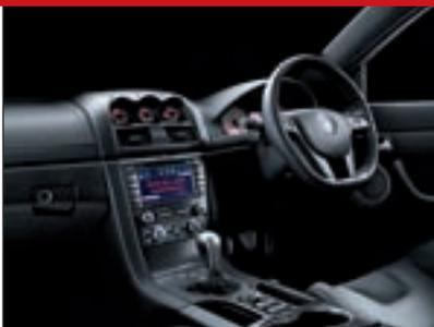
◀ **Performance facia.** The VXR8 steering wheel means business – leather-covered and flat-bottomed with perforated grip zones and remote audio controls. The steering column is reach and rake adjustable too. Other features include alloy pedals, cruise control and dual zone Electronic Climate Control (ECC).
