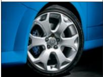
Alloy wheels. The 18-inch six-spoke alloy wheel (left) is standard for Astra VXR, with 225/40 R 18 ultra-low profile tyres. The 19-inch multi-spoke alloys with anthracite inner and 235/35 R 19 tyres (illustrated right) are optional at extra cost.
