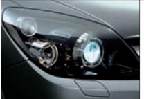
Adaptive Forward Lighting (AFL). The optional lighting system swivels the beams up to 15 degrees for improved vision as you turn a corner. On some models AFL also raises the dipped headlight beam slightly at above 65mph, returning to normal beam automatically as speed is reduced.
