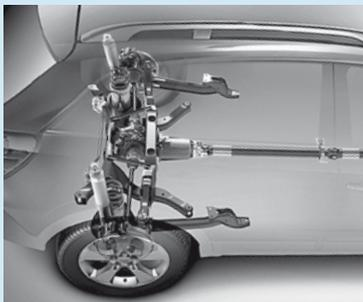
Rear suspension includes automatic self-levelling.
