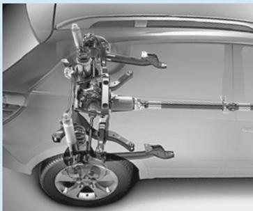
Rear suspension includes automatic self-levelling.
