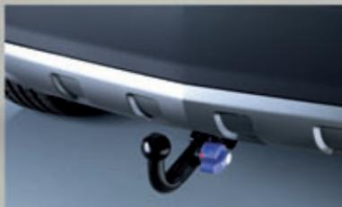
**Detachable coupling tow bar with 12N electrics**. If you want a tow bar coupling that can be removed from your vehicle when you're not towing, this is the choice for you. The coupling is easily mounted and detached for maximum convenience.
