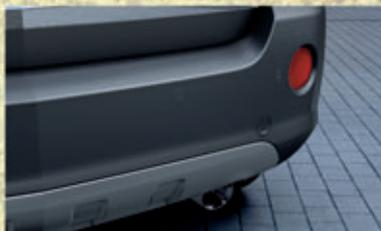
**Parking distance sensors.** Standard on all 4X4 models, this clever Vauxhall system helps safeguard your car when parking. Sensors in the bumpers provide an audible warning when they sense an object behind – or in front of – the vehicle, making it altogether easier to park.
