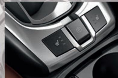
**Heated front seats.** On all models, heating elements in the seat backs and cushions enable the front seats to reach a comfortable temperature in a very short time. There are three separate heat settings.
