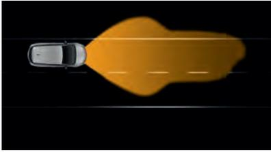
**Motorway light (over 70mph).** 140 metre range, higher and brighter than normal low beam, without dazzle.
