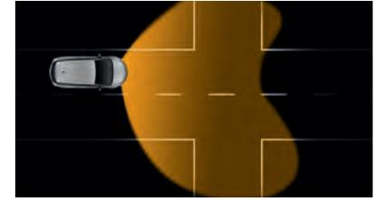
**Pedestrian area light (up to 20mph).** Wider spread of light (an extra eight degrees left and right) illuminates potential hazards.
