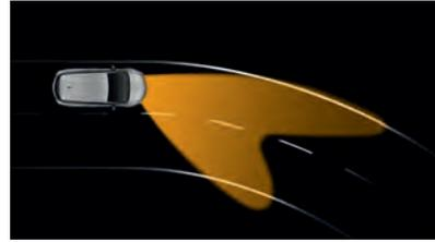
**Dynamic curve light (any speed).** Activated by steering angle and speed, the headlights swivel up to 15 degrees into the curve.
