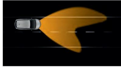
**Country road light (35-70mph).** Wider spread and brighter light than normal low beam. 70 metre range without dazzle.
