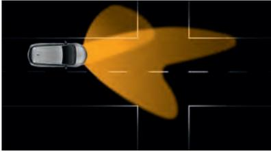
**Static cornering light (up to 25mph, also when reversing).** Throws light 90 degrees left or right for enhanced lateral vision.
