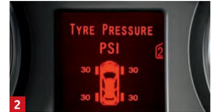
**2. Tyre pressure monitoring system (TPMS).** Monitors the tyre pressure via sensors on the inner sides of the valves and activates a warning display if there is a loss of pressure. Optional at extra cost.
