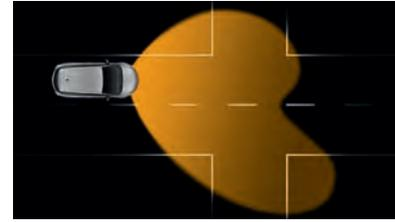
**Town light (20-35mph).** Wider and lower spread of light. Activated by vehicle speed together with street lighting.
