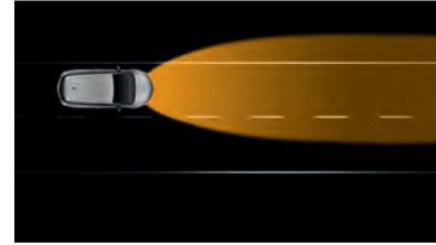
**High beam with assist (over 25mph).** Automatically switches from high to low beam as it detects oncoming or proceeding vehicles.
