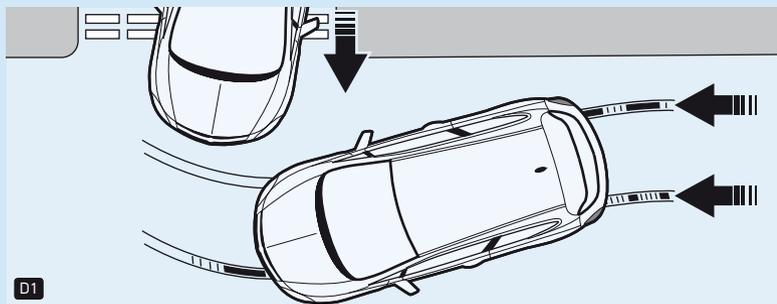
**Anti-lock Braking System (ABS) with Cornering Brake Control (CBC)**
