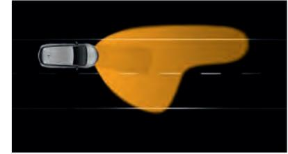
**Adverse weather light (up to 45mph).** Wiper or rain sensor activated for better vision in bad weather conditions.
