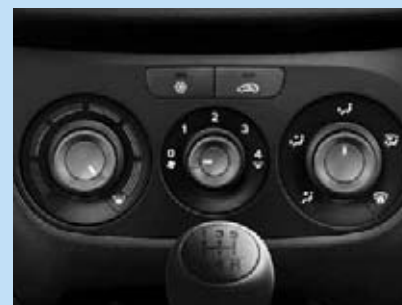
Air conditioning and air recirculation.
