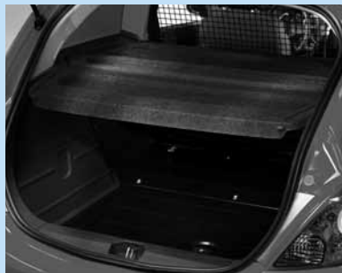
Load compartment cover (four-piece) and upper load restraint mesh.
