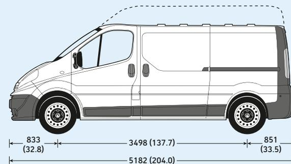
Measurements are shown in millimetres (inches). All heights are shown unladen.
