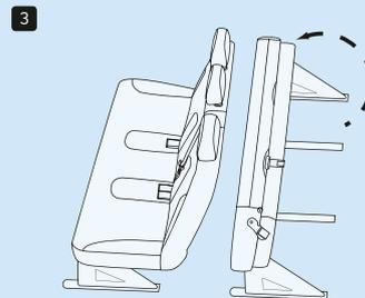
Combi's 'stow and fold' third-row seats (1-3) convert the 9-seat Combi into a six seater with additional luggage space, without having to remove any seats from the vehicle.
