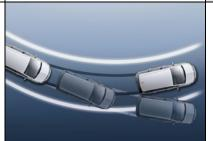
**ESP-plus.** Especially useful on wet roundabouts and greasy roads or whenever a slippery surface catches you out, Electronic Stability Programmeplus (ESP-plus), senses if the car starts to slide on a bend and applies corrective braking to the appropriate wheels to help you regain control.
