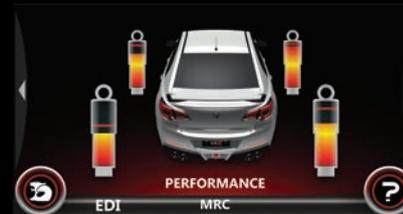
**MRC performance data.** Monitor the performance of the magnetic ride control system in real time.
