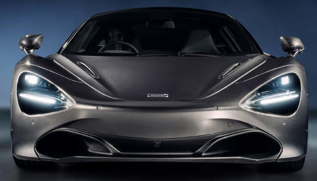
Every curve and form is shaped to manage airflow. Strengthen performance. Ducts within the unique headlights guide air to cool the engine. Fast flowing air is directed through concealed channels in the door skins. So there's no need for visible air intakes. This creates a ruthlessly minimal, shark-like profile.
