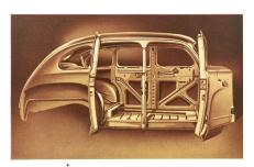
The Ford welded all-steel body with its internal bracing and double steel walled doors is designed as a unit structure of exceptional strength and rigidity. Both you and your passengers enjoy operating quietness with utmost safety and protection.
