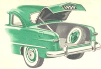
Business or pleasure, you'll appreciate the extra space in Fords' "Deep Deck" Luggage Locker. 22.9 cu. ft. of usable space plus spare wheel room. Rear deck-lid has new "trigger-type" latch—new deck-lid hinges that prevent water, dirt and snow from falling into compartment.
