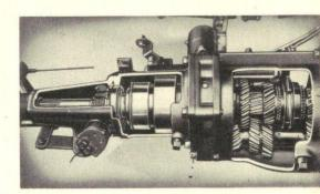
accelerator all the way down and the shift from fourth to direct drive occurs automatically. A "T"-shaped handle control on instrument panel permits overdrive to be "locked-out" when desired.
