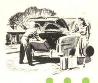
... you'll appreciate the new automatic-releasing decklid holder . . . the new hinges that move the lid up and out of the way to prevent snow and water from dripping into the compartment . . . the fully-lined interior and one-piece rubber floor mat for extra long service and maximum luggage protection.
