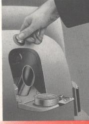
A special lock is provided for the fuel filler cover of the 15 gallon petrol tank, thus ensuring complete security when the vehicle is left unattended.
