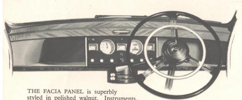
THE FACIA PANEL is superbly styled in polished walnut. Instruments, which include a thermometer, are clear and easy to read, with graduated panel lighting for night driving. Spring steering wheel, with badge in centre, harmonises with the interior. Top of the panel is unpolished, to prevent glare.
