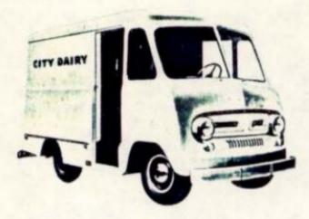
DAIRIES capitalize on Ford Parcel Delivery Chassis' 6-ft. height allowance and low-to-ground door opening for time-saving milk delivery. Adaptable to insulation and refrigeration.
