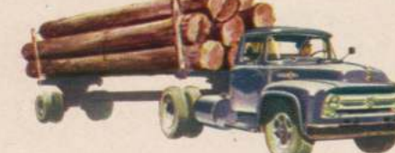
SERIES F-800 BIG JOB for 7½ to 19-ft. bodies. Increased GVW, now 24,000 lbs., for load capacity to 17,445 lbs.* Stronger clutch, new long brake life. 132", 144", 156, 175, 192-in. wbs.
