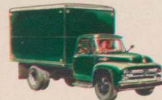
SERIES F-600 for 7½ to 16-ft. bodies. New heavy-duty rear axles. New 18,000-lb. max. GVW for load cap. of 12,980 lbs.* 130", 154, 172-in. wbs.
