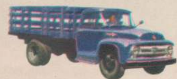
SERIES F-300 for 7½ to 13-ft. bodies. New 15,000-lb. GVW. Improved transmission. Max. load cap. 10,495 lbs.* 130", 154-in., 172 in. wbs.
