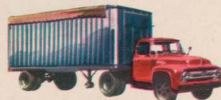
SERIES F-700 BIG JOB for 7½ to 19-ft. bodies. New 21,000-lb. GVW, new stronger axles, new longer-l. 1 q brake linings. Max. load cap. 15,330 lbs.* 132", 144", 156, 175, 192-in. wbs.
