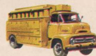
SERIES C-750 BIG JOB for 8 to 16½-ft. bodies. Increased GVW, now 21,000 lbs. New long-life brakes, sturdier rear axle. Power Steering available. 116", 132, 156-in. wbs.
