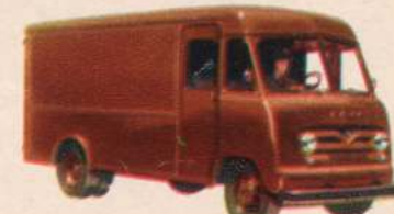
SERIES P-500 Chassis . 130-in. wb. for 10½ to 12½-ft. bodies. New 15,000-lb. GVW. Orscheln hand brake lever standard. Automatic now available.
