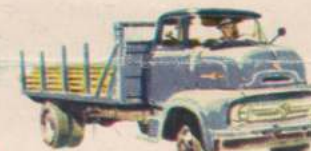
SERIES C-600 for 7½ to 17-ft. bodies. New 18,000-lb. max. GVW, load cap. to 12,935 lbs.* New heavy-duty rear axles. 110", 134, 158-in. wbs.
