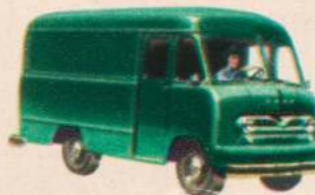
SERIES P-350 Chassis . 104-in. wb. for 7 to 9-ft. bodies. 122-in. wb. for 9½ to 11½-ft. bodies. New 8,000-lb. GVW. Automatic Drive available.
