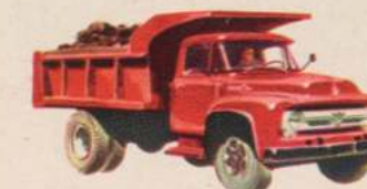
SERIES F-900 BIG JOB for 7½ to 19-ft. bodies. New 29,000-lb. GVW boosts load capacity to 22,180 lbs.* New, more durable clutch and brakes. 132", 144", 156, 175, 192-in. wbs.
