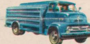
SERIES F-700 BIG JOB for 7½ to 19-ft. bodies. New 21,000-lb. GVW, new stronger axles, new longer-l. 1 q brake linings. Max. load cap. 15,330 lbs.* 132", 144", 156, 175, 192-in. wbs.
