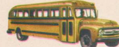
SERIES B-700 for up to 66-passenger bodies. New 21,000-lb. GVW. New 245-in. wb. New sturdier axles, longer-lasting brakes.
