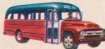
SERIES B-500 for up to 36-passenger bodies. New 15,000-lb. GVW. New, stronger 4-speed transmission. 154-in. wb.
