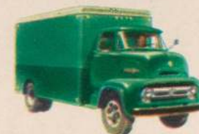
SERIES C-700 BIG JOB for 8 to 16½-ft. bodies. New 21,000-lb. GVW boosts load capacity to 15,030 lbs.* New stronger rear axle, longer-lasting brakes. 116", 132, 156-in. wbs.
