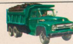
NEW SERIES T-750 BIG JOB for 10 to 19-ft. bodies. Max. GVW of 36,000 lbs. for load capacity to 26,865 lbs.* Power Steering standard. Vacuum-powered or air-over-hydraulic brakes. 144", 156, 175, 192-in. wbs.
