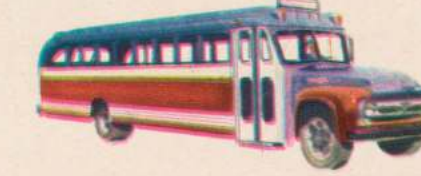
SERIES B-750 for up to 66-passenger bodies. New 21,000-lb. GVW. New 245-in. wb. New sturdier axles, longer-lasting brakes.
