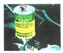
NEW MULTI-LUBER is optional on all '56 Monarch models. By touching a button on the instrument panel you automatically lubricate all front suspension and steering points.
