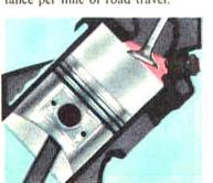
NEW COMBUSTION CHAM-BER DESIGN creates maximum turbulence for smoother, faster burning of fuel. Intake and exhaust breathing at all speeds is improved by high-lift valves and larger ports.
