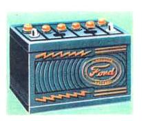
NEW 12-VOLT SYSTEM provides extra electrical power for the heavy demands of today's driving. It turns the starter twice as fast, for more reliable starting in winter weather.
