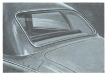
SAFE, CONFIDENT REVERSING Rear window is extra large and curved to blend with the contour of the body. The driver has an excellent rearward view. Filler cap of the 13-gallon (59-litre) fuel tank is concealed.
