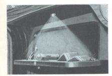
ROUTE-FINDING EASIER Lid of the glove box on the passenger's side hinges downwards to form a useful shelf for map-reading. A lamp illuminates the shelf from above.
