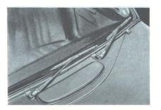
DUAL WINDSHIELD WIPERS Driving vision is always clear and safe as twin wipers sweep the windshield in wide arcs. They are selfparking, too! Windshield washing equipment is also a standard fitment.
