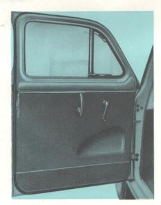
The wide fully trimmed front doors include parcel pockets, wind-up windows and nodraught pivoted ventilators are adjustable to suit all weather conditions.
