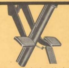
New suspended clutch and brake pedals eliminate toeboard holes for a tighter sealed cab.
