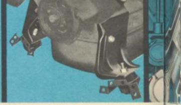
New 2-point front engine mounts soak up vibration—anchor front of engine to provide greater stability and smoother, quieter engine operation. (Six shown.) Note that the state of the land of the lan
