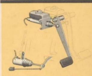
New hydraulic clutch works like a hydraulic brake—requires less foot pressure, makes shifting easier.
